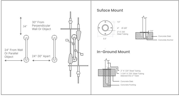
Most of our units are suitable for either surface mount, in which case the bike racks will have a flange for easy mounting to the ground. See suggested fasteners below. Or in-ground installation, in which case the bike racks will have an approximate 10" extension for embedding in concrete beneath the surface.
