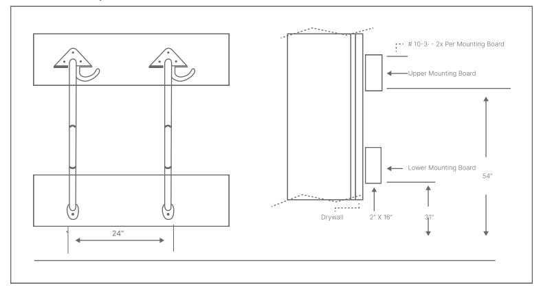
Stud walls are typically 16" on center. Stagger height by 10" for 16" on center installation (use lag screw indicated below). For 24" spacing (no bike lifting), see below.
