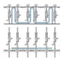
Each bike has equal access to the rack. Locking the bike frame and front wheel with a U-lock is easy. With the bikes held apart there is little interference between handlebars and petals.
