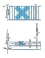
It's not enough to lock just the front wheel. When used as intended, this design prohibits the use of the U-lock on the bike frame.
