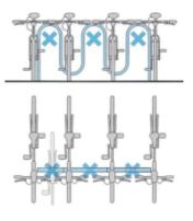
Better than it's predecessor, but the design creates it's own set of problems. Difficulty in bike placement and access can cause this rack to become full at two thirds of it's intended capacity.
